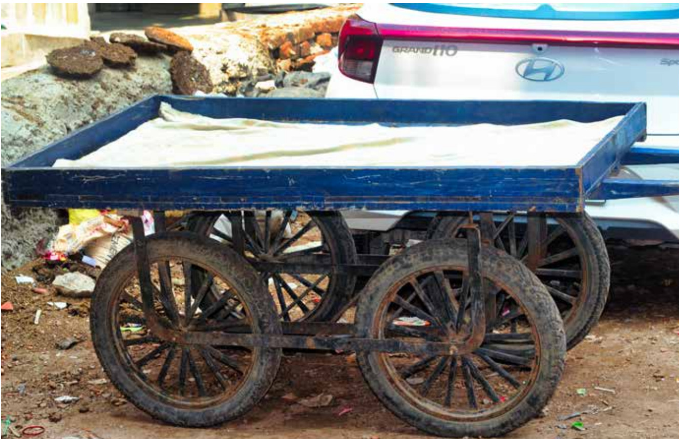
The broad wheel base carts provided under one batch of SMILE Carts. Beneficiaries recommended similar broad wheel base carts be provided in the future and not the narrow wheel base carts being provided currently. The broad wheel carts are more sturdy and easy to manoeuvre on ill prepared roads.
